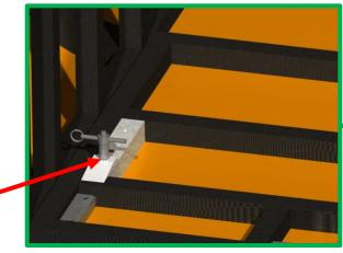
Adjustable stops and fuselage frame position payload
