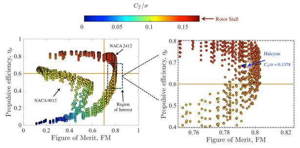
Using blade element momentum theory, the performance of 5,500 independent fixedpitch blade designs was assessed in hover and cruise modes to determine the optimum blade twist and taper. Hover efficiency was prioritized to reduce the vehicle empty weight while preserving sufficient stall margins and propulsive efficiency.
