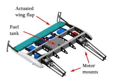
*Halcyon's* wings house the motors, motor mounts, fuel tanks, and wing flaps.
