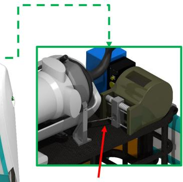
Hoist cable passes through roller box to payload
